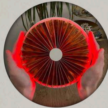
Indicative Light Neopixel ring shows phase via customisable gradient
